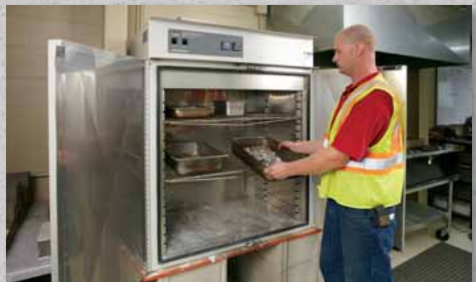
Aggregate Moisture Test
