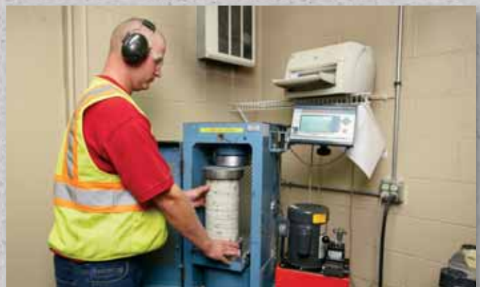
Concrete Cylinder Compressive Strengths Test
